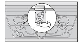
■ Unscrew the wing nuts and lower the top heating element.
